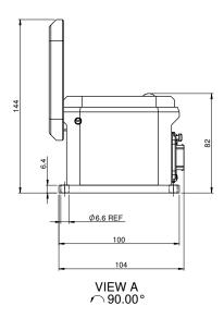
Helios Plus - Profinet / Helios Plus - EtherNet/IP / Helios Plus - EtherCAT with Cover Closed
