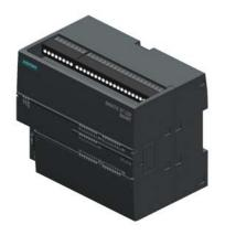
\*\*\* spare part \*\*\* SIMATIC S7-200 SMART, CPU ST40, CPU, DC/DC/DC, onboard I/O: 24 DI 24 V DC; 16 DO 24 V DC; power supply: DC 20.4-28.8V DC, program/data memory 40 KB
