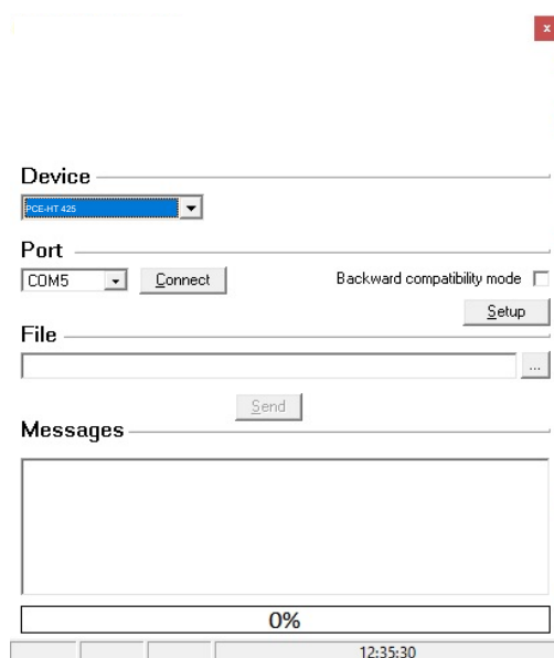
Fig. 30. View of the program to upgrade the firmware.
