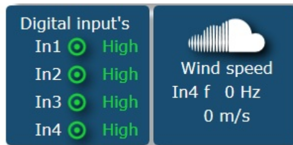
Fig. 35. Tiles of the web server presenting the state of binary inputs
