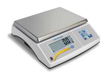
Reasonablypriced Benchtop Scale up to 30 kg / accuracy down to 0.05 g / operation by battery possible / bi-directional RS232 interface /platform size  $300 \times 210 \text{ mm}$  / optionally purchasable: LAN, Wi-Fi, 4-20mA, 0-10 V or 3 potential-free contacts
