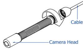
Figure 8. Assembly/Disassembly Camera
