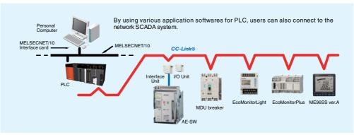
The length of the cable for interface unit is 2m.
