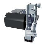
The closing spring is charged by an electric motor. When the breaker is closed, the spring is charged automatically (ON-charge method). The closing coil (CC) is required to remotely close the breaker, and the shunt trip device is required to remotely open the breaker.
