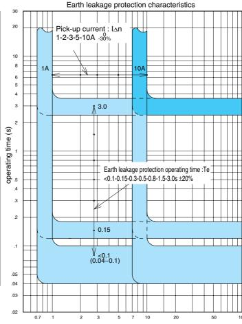
Earth leakage current (A)
