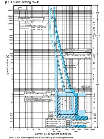
current (% of current setting Ir) Note 1: LTD operating time tLTD is calculated by the following equations
