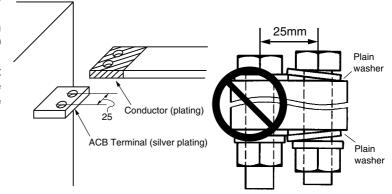
Since fault current flowing through the conductors causes large electromagnetic forces, the conductors should be secured firmly, using the values in the below table as a reference. Max. distance between fixing support and ACB bus bar should be less than 200mm.
