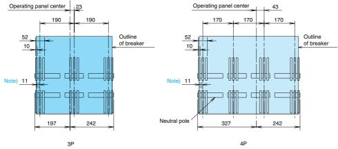
Note) Spacers are not required when fastening connecting conductors (T10). The necessary contact area can be obtained with ACB terminal bent by tightening the screw.
