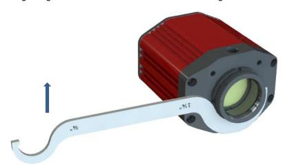
Figure 8 Tightening the Adjustable C-mount Adapter
