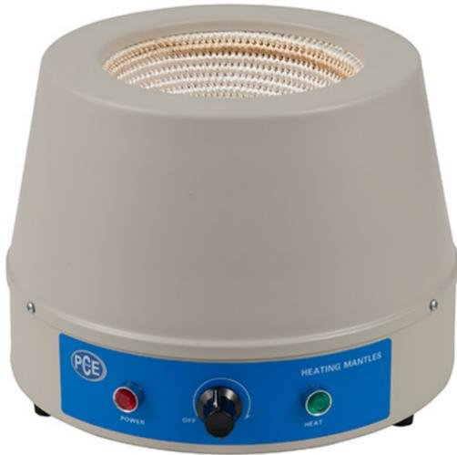
**HeatingMantle for 500 ml round-bottom flask / stepless variable (rotaryswitch) / with 250 watt power / with integrated controller / temperature range 0... 450 °C**
