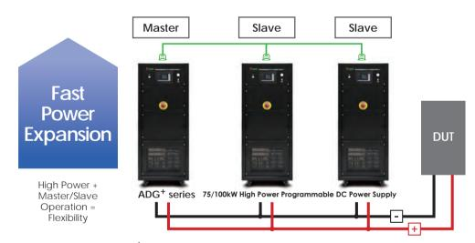
The output power of the ADG<sup>+</sup> series is up to 100kW per unit, which can be expanded to 300kW through simple master-slave operation (max. 3 units). User can simply operate the master unit, the slave unit will receive and reply the data accordingly and equally share the load current. ADG+ series is one of the few high-power DC power supply with parallel feature on the market. The availability for single-unit and parallel operation provides greater flexibility for application.
