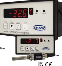
Model AcuTrak accepts a universal supply input of 90-250 V AC (a 24 V DC option is also available). The linear 4-20 mA signal retransmission is adjustable and can be configured across the range of the dewpoint transmitter. Various dewpoint ranges are available covering an overall range from -120 °C to +20 °C (-184 °F to +68 °F) dewpoint.
