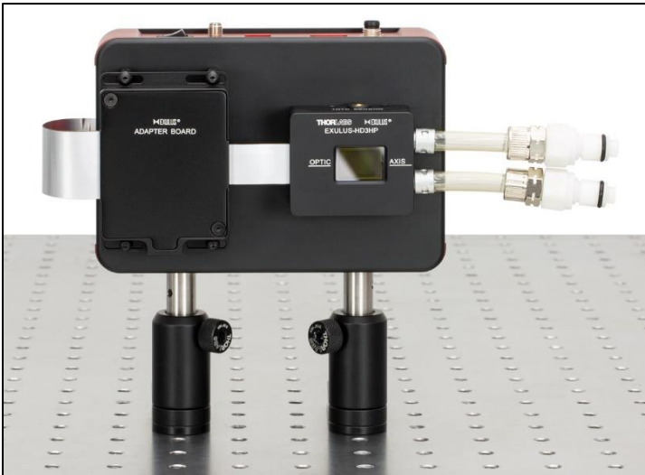
Figure 25 Post Mounting the High-Power SLM, All-in-One Mode
