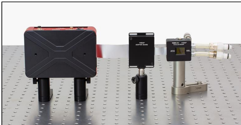
Figure 26 Post Mounting the High-Power SLM, Separate-Panel Mode
