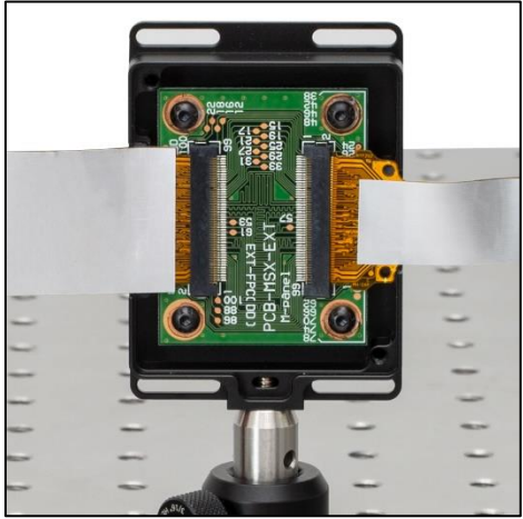
Figure 33 Aligned FPCs for Both Board and Panel Sides
