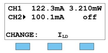
Now, the main parameter (here ILD in mA) can be adjusted by means of the tuning knob. Pressing the keys completes the procedure.
