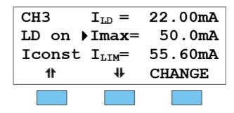
Pressing the soft key **CHANGE** activates the tuning knob to change the selected parameter. If the parameter is only to toggle (e.g., polarity of the laser diode), the function of the soft keys will change:
