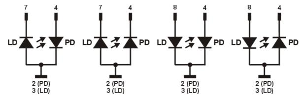
LD - Laser Diode; PD - Photo (Monitor) Diode
