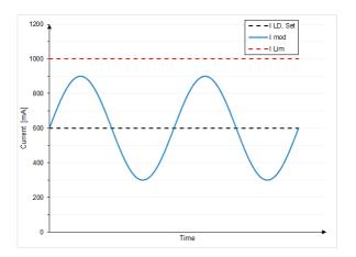
The diagrams below show settings that lead to laser current clipping:
