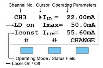
Only three parameters can be shown at a time, so there is a scroll function. All parameters are sorted in a virtual list, which can be run through with the cursor:
