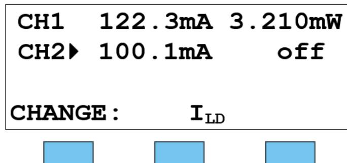
Now, the main parameter (here  $I_{LD}$  in mA) can be adjusted by means of the tuning knob.
