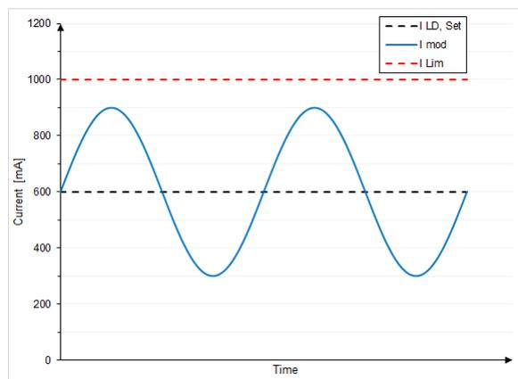
The diagrams below show settings that lead to laser current clipping:
