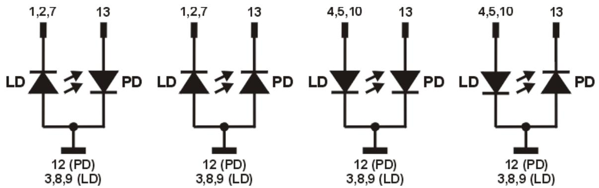
*LD - Laser Diode; PD - Photo (Monitor) Diode*
