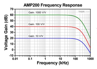
This graph shows calculated data using an input source with 50  $\Omega$  and 100 pF.
