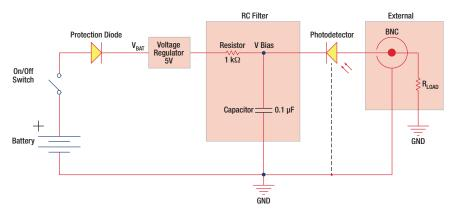
Figure 2 Basic DET Circuit
