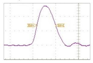
Figure 4  $T_r = 122 \text{ ps. } T_f = 170 \text{ ps } @ 20/80\%$
