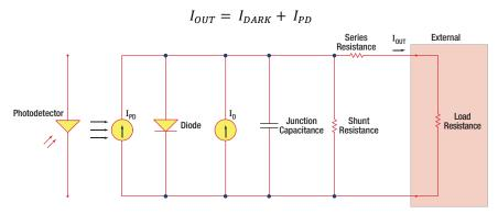
Figure 1 Photodiode Model
