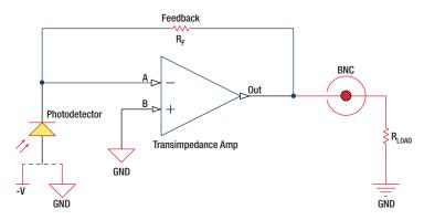
Figure 3 Amplified Detector
