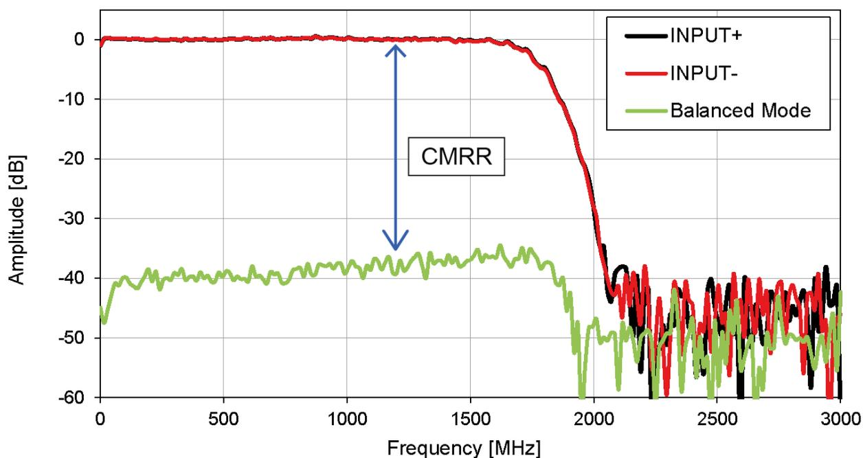
**PDB480C-AC: Typical MONITOR OUTPUT Frequency Response**
