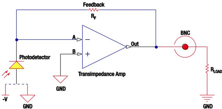
Figure 3 Amplified Detector
