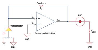
Figure 3 Amplified Detector
