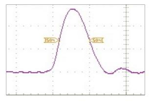
Figure 4 T<sub>r</sub> = 122 ps. T<sub>f</sub> = 170 ps @ 20/80%
