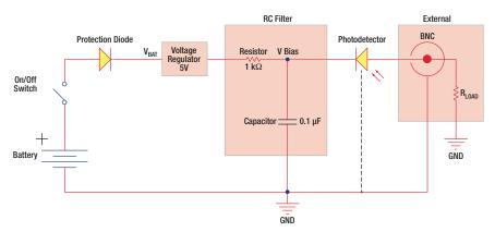
Figure 2 Basic DET Circuit
