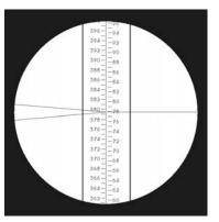
Example above: Staff reading 77cm Micrometer reading 0.556cm Height 77.556cm
