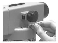
Fig.5 Adjusting the circular bubble.
