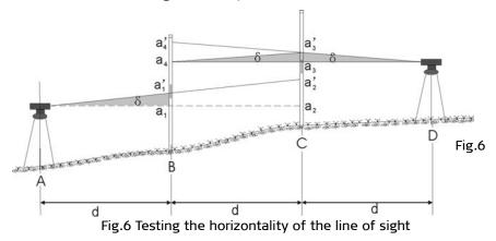
In 7.3.2 the tolerance of 2mm in 30m is a practical value for routine leveling with the instrument. If necessary, however, a customer can make a more precise adjustment.
