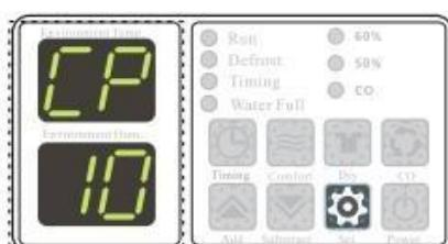
Press 10 seconds continuously to enter the internal parameter setting mode
