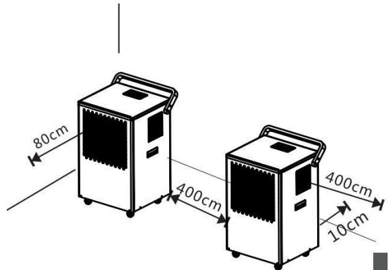
[The best position is placed by opposite instead of in the same line. Otherwise the right side dehumidifier will detect more dry air generated by the left side dehumidifier instead of the room's wet air.]
