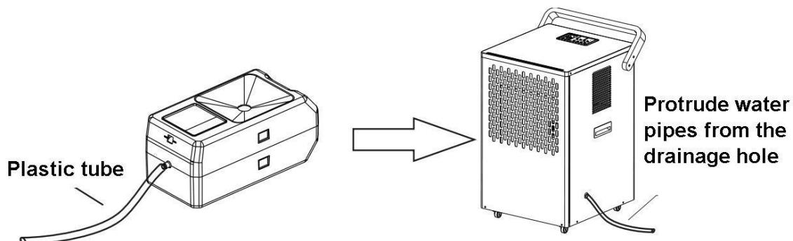
First, insert the drainage hose into the drainage port on the side of the water tank, and then put the
