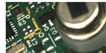
Imaging Sensor Circuit Board inspected by classic microscope
