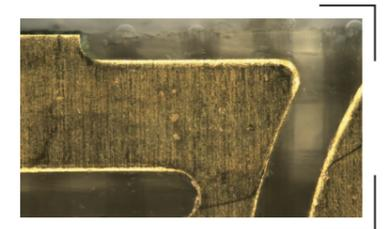
Ring Light illumination with glare removal (details on the edges now visible)
