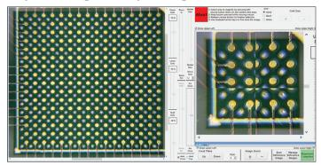
A high definition Vision Overlay System uses bright white LEDs with independent intensity control to provide precise distinction of pads and solder ball or leads.
