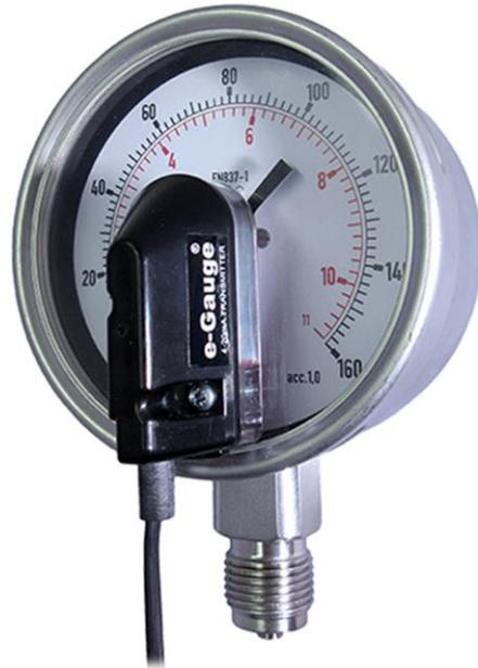
**e-Gauge-lite** is used to convert pressure or temperature gauges to pressure and temperature transmitters, it reads the position of the pointer on any 100mm or 160mm DIN cased analogue gauge to give a 4-20mA output.
