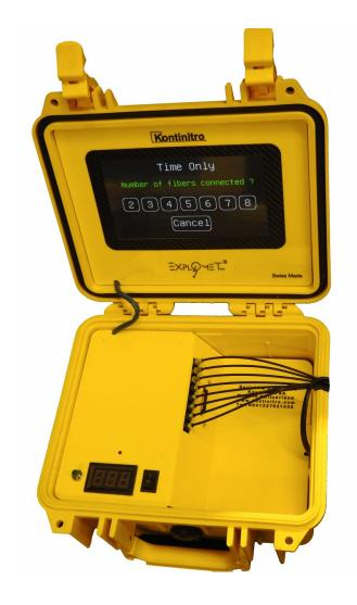
The Explomet<sup>3</sup> is designed for V.O.D. measurements of explosives, detonators, detonating cords, fuels, oxidizers, etc. in the laboratory, in the field and in the <u>blast hole</u>.
