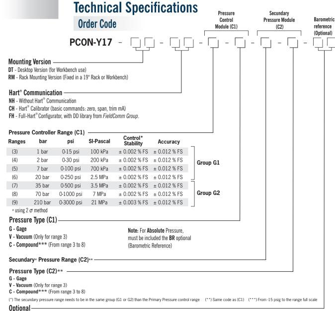
**BR** - Barometric Reference to measure and emulate absolute pressure Accuracy 0.16 mmHg / 0.2 mbar
