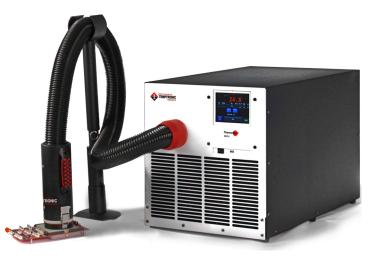
User-programmable temperatures, graphing, and data logging are established through the controller's touch-screen or remote communications. The system provides fast and precise transitions of temperature at the IC, even with variations in device power, and can be used with Temptronic's proven DUT Control technology using an imbedded diode or external thermocouple.
