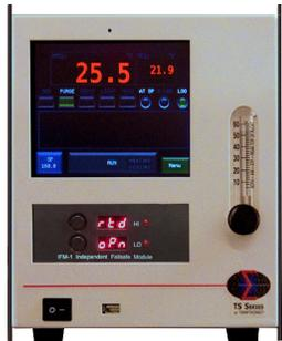
Optional Dry Nitrogen Purge Systems eliminate moisture and/or oxygen from the test environment.
