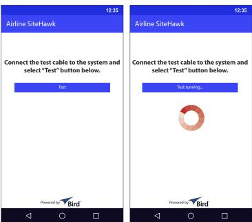
When the test is complete, the result is displayed on the screen. If the test passes, the system's VSWR is below the threshold set for the test. If the test fails, the VSWR is above the threshold set for the test. See Figure 7.
