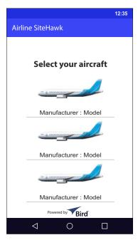
The FlightHawk-AV contains predefined configurations for testing an aircraft's communications or navigation systems. Each system on the aircraft will be listed, the technician chooses the appropriate system by tapping the screen. See <u>Figure 5</u>.
