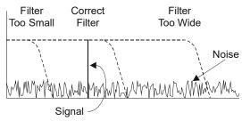
Except for average power and VSWR measurements, all WPS measurements rely on a variable video filter to improve accuracy. This filter can be set to either 4.5 kHz, 400 kHz, or full bandwidth (10000kHz). It should be as narrow as possible while still being larger than the demodulated signal bandwidth (video bandwidth). Narrowing the filter limits the noise contribution caused by interfering signals. Listed below are some common modulation schemes and the appropriate video filter.
