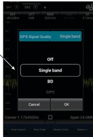
GPS Signal Quality Measurement Turns on Both Preamps
