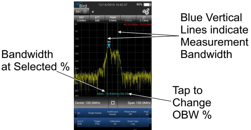
The calculated occupied bandwidth represents the user specified percent of the total power of the displayed span.
