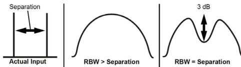
As the RBW decreases, more and more resolution between the two signals will be seen, and consequently, one full sweep over the set span will take longer to complete. It is important to note, however, that RBW can be too narrow in some instances. For example, if the RBW is not wide enough to include the sidebands of a modulated signal, the spectrum analyzer will display an inaccurate measurement.
