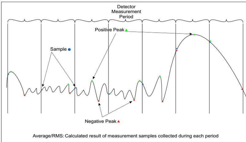
For low-level signal detection, setting the Detector to Average or RMS displays the average of the raw data collected for each display pixel. This is recommended for noise-reduction, since averaging the multiple raw data samples collected for each data point makes the resulting measurement less sensitive to noise. The number of raw data samples collected by Bird's SignalHawk is controlled by a combination of the RBW, VBW, and the frequency span settings.
