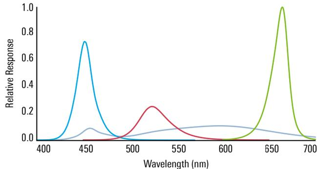
Figure 7. The large light source provides peak emission at 453 nm for blue, 523 nm for green, 660 nm for red. White is nominally at a 4000 K color temperature.
