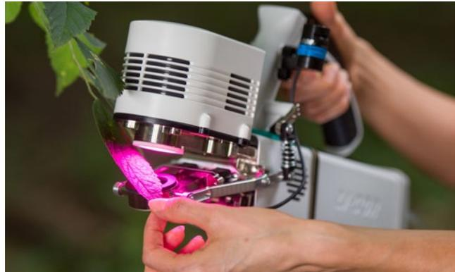
The Multiphase Flash™ Fluorometer chamber (6800-01A) can function as full fluorometer or simple light source. The fluorometer chamber enables the Dynamic Assimilation™ Technique.
