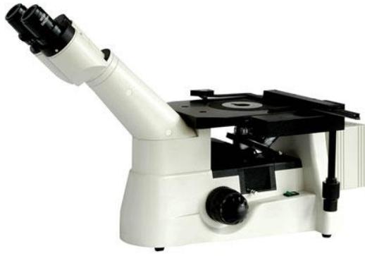
This series microscope is widely used in observation & analysis of metallurgical organization in the Mechanical industry, Research of Geological & Mineral department and viewing & measuring crystal, integrate circuit, microelectronics, etc in Electronic industry. It is the first choice of Factories, Academy, Scientific research organization contrast image. Novel figure and superior crafts manship keep abreast of the tidal current much more.
