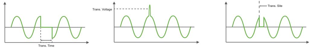
Through the Transient feature, user can have more control over the waveform by inserting disturbance at user-defined locations with user-defined drop/rise range. This is a useful feature to simulate different pre-compliance tests and various types of power line disturbance, such as surge, sag, spike and dropout, for immunity tests.
