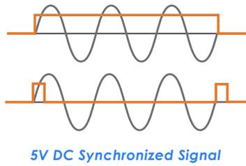
AFV-P series provides two types of synchronized signal. It can either deliver a 5V DC signal continuously when the product output is on or deliver a 5V DC pulse signal every time there is a change on the product output. This feature makes AFV-P series an ideal AC source when applying with automatic test systems.
