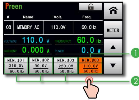
To create a complex sequence on the HMI is no longer a difficult task for AFV-P series. The 5 inches touch screen provides users a clear display and an easy set up. AFV-P series can display 4 shortcuts of Memory Sets, and the voltage and frequency setting of each Memory Sets can be clearly read. The user can quickly switch the output by selecting the shortcuts.
