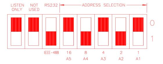
Figure 8-2: GPIB Address Selection Switch
