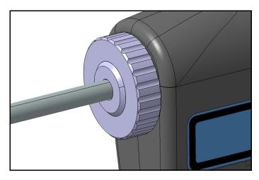
Wheel for the axial adjustment to vary the angle of view of 175 ° clockwise and counterclockwise. In this way, the viewing direction can be axially adjusted, without the endoscope with the handle must be rotated.
