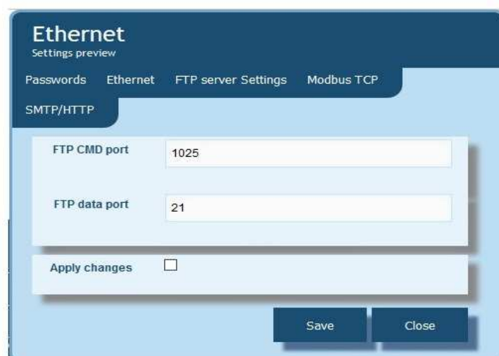
Fig.18 View of FTP ports configuration window
