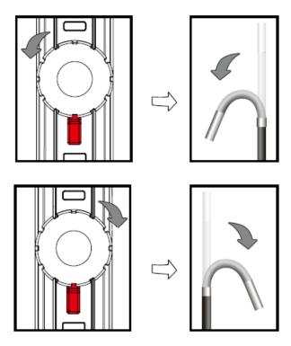
2. You can lock the pivoting angle of the camera head by using the red locking lever. To lock the camera head, carefully push the lever clockwise all the way to the stop. To unlock the camera head carefully push the lever counter-clockwise, until it reaches its starting point.
