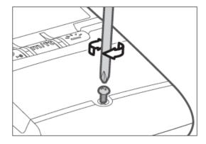
The battery compartment of the cable measuring device is located at the front, right below the function keys. To open it, you have to loosen a screw first. After that, you can open the battery compartment and replace the batteries.
