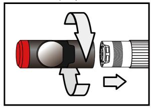
Step 4: Align the lateral LED opening of the mirror attachment in a way that the LEDs are uncovered. Step 5: Turn the assembly ring upwards in order to fix the mirror attachment.
