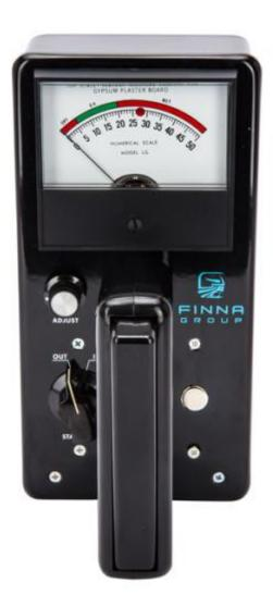
This single range instrument uses the Radio Frequency Capacitance Method to measure the moisture content of Gypsum Wallboard. Color Coded direct reading dial for fast comparison. Has a range of 0 to 25% and is operated from a single rechargeable NiMH battery. It gives the operator an average moisture content down to a penetration of one inch. The LG uses Stainless Steel Buttons that make contact with the board. Complete with a Carrying Case, NiMH Battery and Operating Instructions Book.
