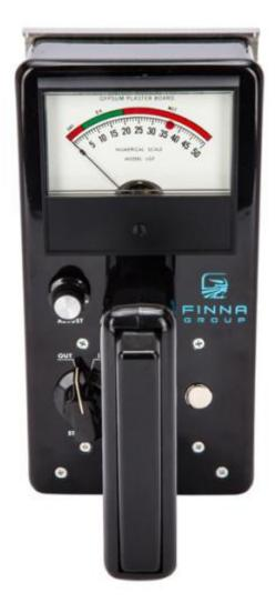
This instrument is similar to the LG instrument, except that it has a stainless steel flat plate electrode. Excellent for testing Gypsum Wallboard as it moves or in stacks. Measures the moisture in the Gypsum plasterboard 1/4 inch to 3/4 inch thick. Color Coded direct reading dial for fast comparison. Can be used to check the moisture distribution pattern on the board-along the length or width. Complete with a Carrying Case, NiMH Battery and Operating Instructions Book.
