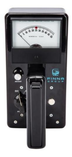
The Model V veneer moisture meter is calibrated for 48 hard and soft woods in the 0 to 25% moisture range and has dials for specific woods. Accurate to 1/8" penetration. Complete with rechargeable NiCad Battery, Carrying Case and Operating Instructions Book.
