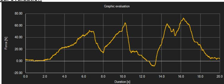
In the graphical evaluation area, the selected unit (force or pressure) is shown on the y axis and the time lapse is shown on the x axis. When moving the cursor over a dot on the displayed line, a small information box will appear after a short time, showing the data (time and unit) of the currently selected measurement value. This value can be selected from the chart by double-clicking on it.
