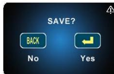
Press **YES** by
