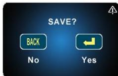
Press **YES** by
