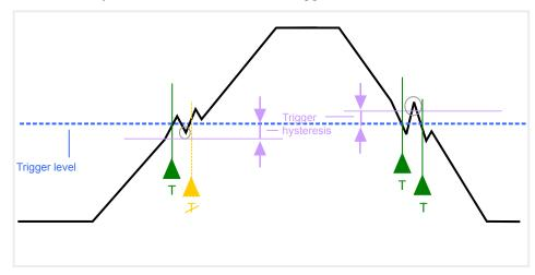
Figure 7-37: Effects of the trigger hysteresis
