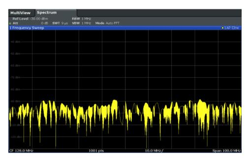
Figure 7-1: Sine wave signal with low S/N ratio
