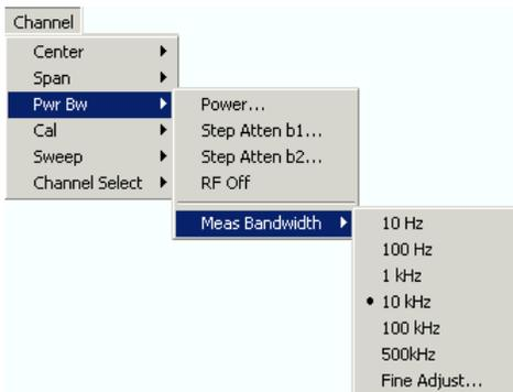
*Fine Adjust...* opens a dialog to modify the selected measurement bandwidth and the selectivity of the IF filter.
