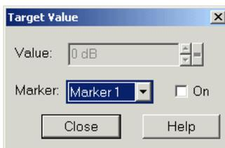
It is possible to define up to ten different target values for each trace and assign them to the markers no. 1 to 10. The input fields in the *Target Search* dialog are used to select the markers and define the associated search ranges:
