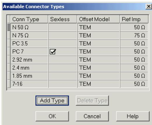
The list shows the available connector types with their name (*Conn Type*), polarity (*Sexless*) and reference impedance (*Ref Imp*). The *Offset Model* describes the mode of wave propagation in the transmission lines of the standards associated with the connector type. The buttons below are used to add and delete user-defined connector types. Deleting a connector type will also delete all calibration or adapter kits assigned to it.
