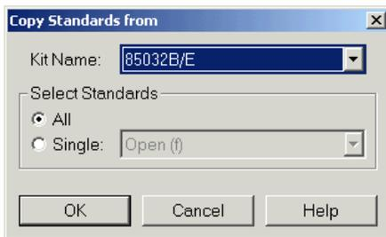
In the dialog, it is possible to select one of the calibration kits in use (*Kit Name*) and select either all or a single standard to be copied. A calibration kit may only contain a single standard of each type.
