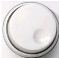
Turning the rotary knob is equivalent to the action of the cursor up and down keys. Turn the knob in order to
