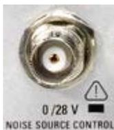
Conventional noise sources require a voltage of +28 V in order to be switched on and 0 V to be switched off. The output supports a maximum load of 100 mA.
