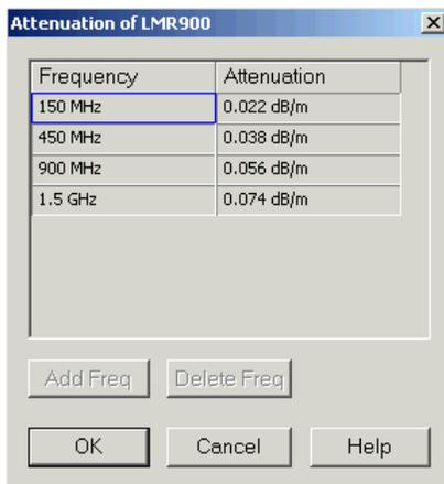
For user-defined cables, the *Frequency* and *Attenuation* columns in the dialog are editable. The frequency dependence can be defined in two alternative ways:
