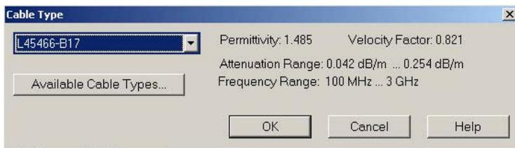
The pull-down list in the *Cable Type* dialog contains an ideal air line (with a relative permittivity of 1, a corresponding velocity factor of 1, and zero attenuation) and a wide range of standard cable types. Click *Available Cable Types* to open a second dialog where you can view the parameters of the predefined cable types and add new types.
