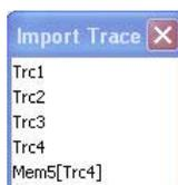
The box contains all data or memory traces of the active channel. As soon as a trace is selected, the *Properties of Imported Segments* dialog with further global import options is opened.
