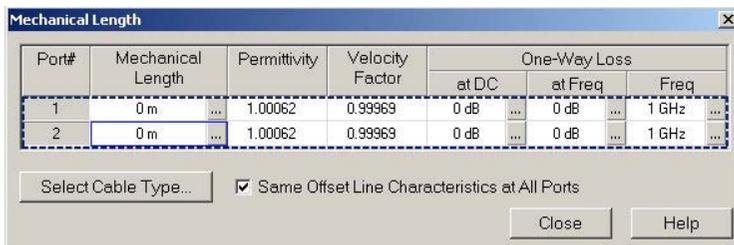
The *Mechanical Length* dialog contains the three editable columns *Mech. Length*, *Permittivity* ( $\epsilon_r$ ) and *Velocity Fact*  $1/\sqrt{\epsilon_r}$ ; see *Offset parameters: Definition* above. Permittivity and velocity factor are coupled parameters. The dialog provides the following additional control elements:
