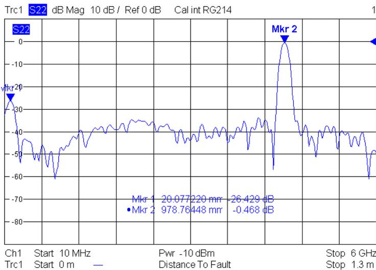
The parameters of the impulse response and frequency-domain representation are related due to the mathematical properties of the time-domain transform. In practice, this means that the sweep points may have to be adjusted to the length of the transmission line and the expected distance-to-fault:
