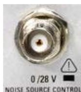
Conventional noise sources require a voltage of +28 V in order to be switched on and 0 V to be switched off. The output supports a maximum load of 100 mA.
