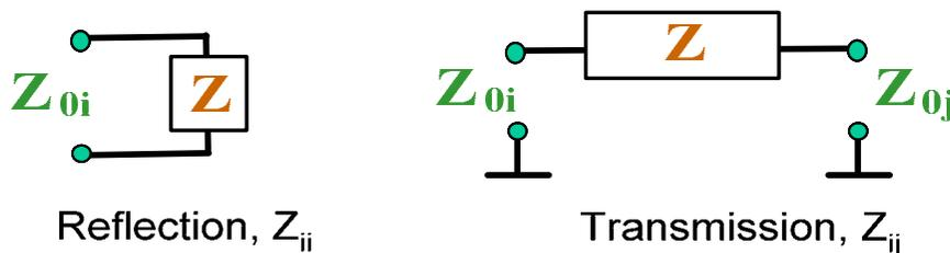
The analyzer converts a **single** measured S-parameter to determine the corresponding converted impedance. As a result, converted Z-parameters cannot completely describe general n-port DUTs:
