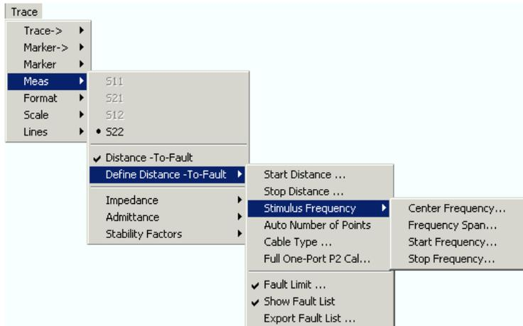
The stimulus frequency settings that the R&S ZVL uses for the distance-to-fault measurement are identical with the general *Channel – Stimulus* settings. Previous settings are not restored when the distance-to-fault measurement is switched off.
