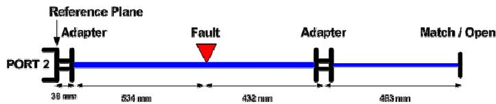
To prepare the distance-to-fault measurement, first perform a full one-port calibration at PORT 2:
