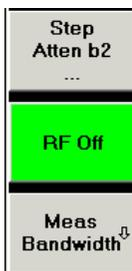
The softkey bar shows up to 7 commands of the active menu indicated above softkey no. 1. The figure above shows the upper part of the softkey bar corresponding to the *Trace – Meas* submenu. Pressing the key to the right of a softkey directly activates a submenu, calls up the numeric entry bar or a dialog or initiates an action. See *Softkey Bar* in the introductory chapter for more information.
