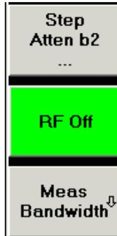
Up to 7 softkeys, each corresponding to a command of the active menu. The function of the softkeys and their labels are strictly equivalent to the corresponding menu commands.
