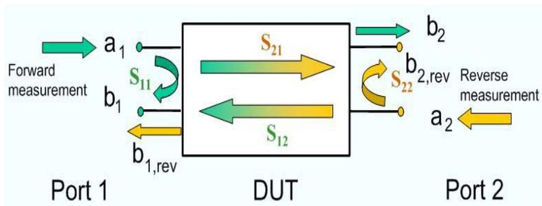
The S-parameters are the basic measured quantities of a network analyzer. They describe how the DUT modifies a signal that is transmitted or reflected in forward or reverse direction. S-parameters are expressed as  $S_{\langle out \rangle \langle in \rangle}$ , where  $\langle out \rangle$  and  $\langle in \rangle$  denote the output and input port numbers of the DUT.
