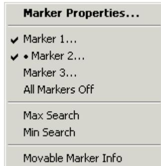
*Movable Marker Info* allows the marker info field to be placed to any position in the diagram area. The remaining settings correspond to the most common commands in the *Trace – Marker* and *Trace – Search* menus.
