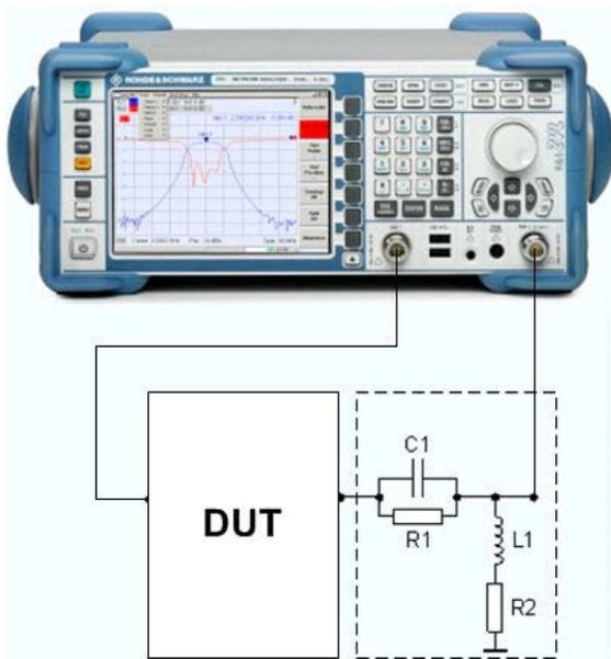
The idea of virtual embedding is to simulate the matching network and avoid using physical circuitry so that the analyzer ports can be directly connected to the input and output ports of the DUT. The matching circuit is taken into account numerically. The analyzer measures the DUT alone but provides the characteristics of the DUT, including the desired matching circuit. This method provides a number of advantages:
