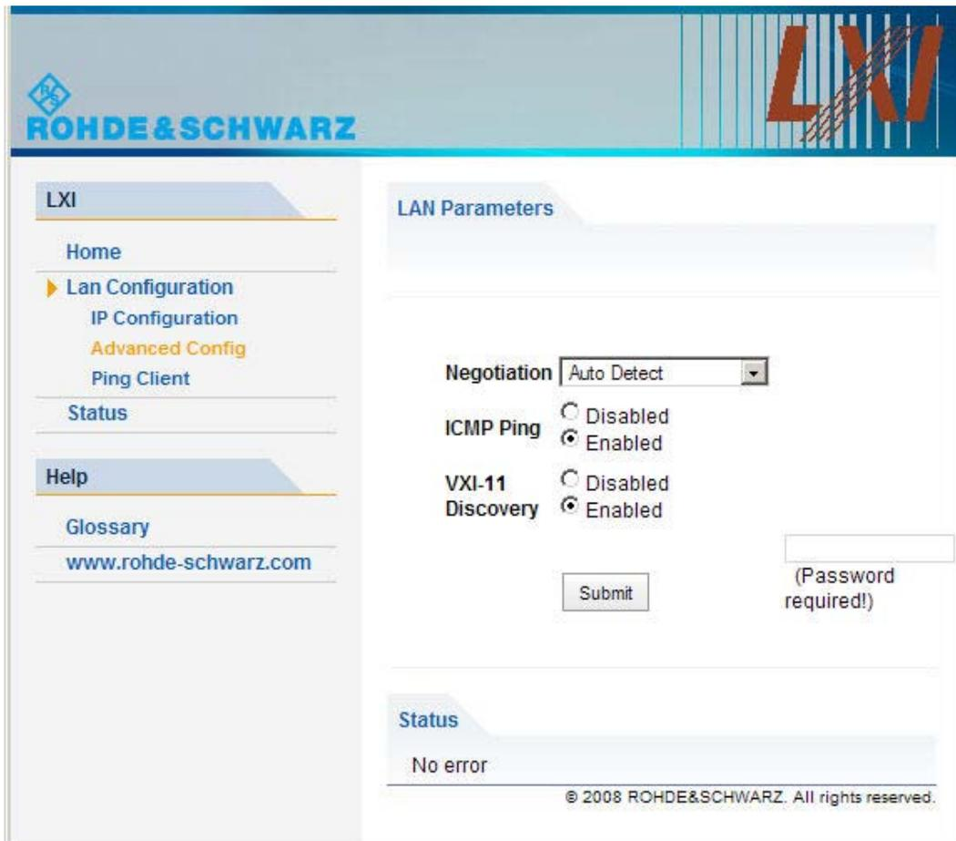
The screenshot shows the LXI LAN Configuration GUI. The left sidebar contains a navigation menu with the following items: LXI, Home, Lan Configuration (with a sub-menu for IP Configuration and Advanced Config), Ping Client, Status, Help, Glossary, and www.rohde-schwarz.com. The main content area is titled 'LAN Parameters' and contains the following settings:
