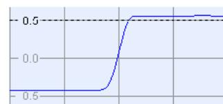
The step response is recommended for impedance measurements and for the analysis of discontinuities (especially inductive and capacitive discontinuities). The impulse response has an unambiguous magnitude and is therefore recommended for most other applications.
