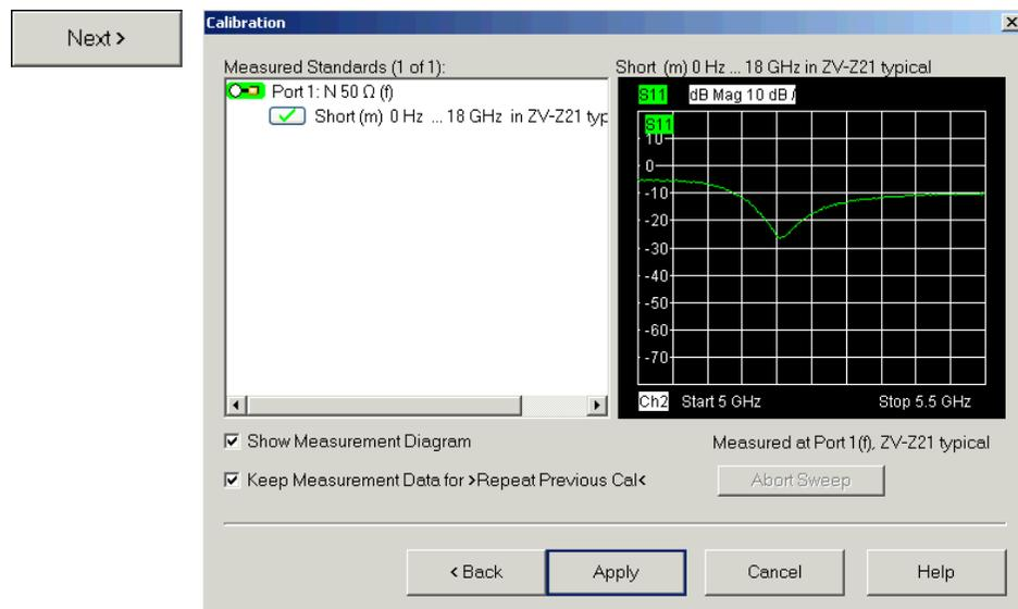
The next dialog of the calibration wizard shows that only a single calibration standard needs to be measured.
