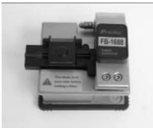
4. Slide the blade carriage to rear side of the cleaver. The fiber will be cleaved.
