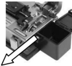
2. Insert the fiber cable into the correct groove with the end of the fiber coating.
