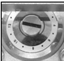
2. Rotate the blade to the next position by pressing its side or edge with cotton swab.
