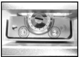
3. Cut fiber for test the performance of cleaver, if not qualify adjust the blade again until optimal the quality.
