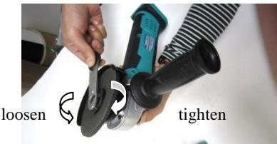
**Attention! Actuate the spindle lock button only when the grinder spindle is at a standstill. Otherwise, the machine may become damaged.**
