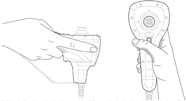
Hold the device with one hand and use your thumb for operating the joystick and the function keys. With your index finger, you can use the boost key.
