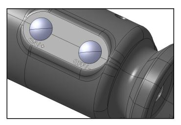
Buttons for switching on and off or adjust the Econoscopes LED intensity over seven levels of brightness. Press the Off button for five seconds to turn off the illumination. The red LED will flash briefly, the button can be released and the Econoscope turns off.
