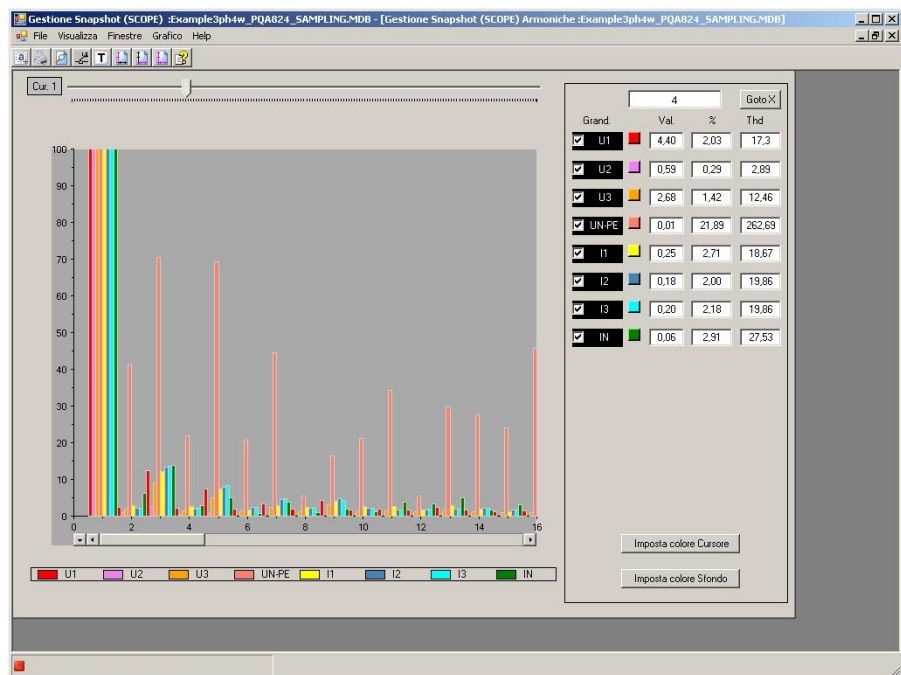
Histogram screen of harmonic analysis of voltage and currents up to 49° order
