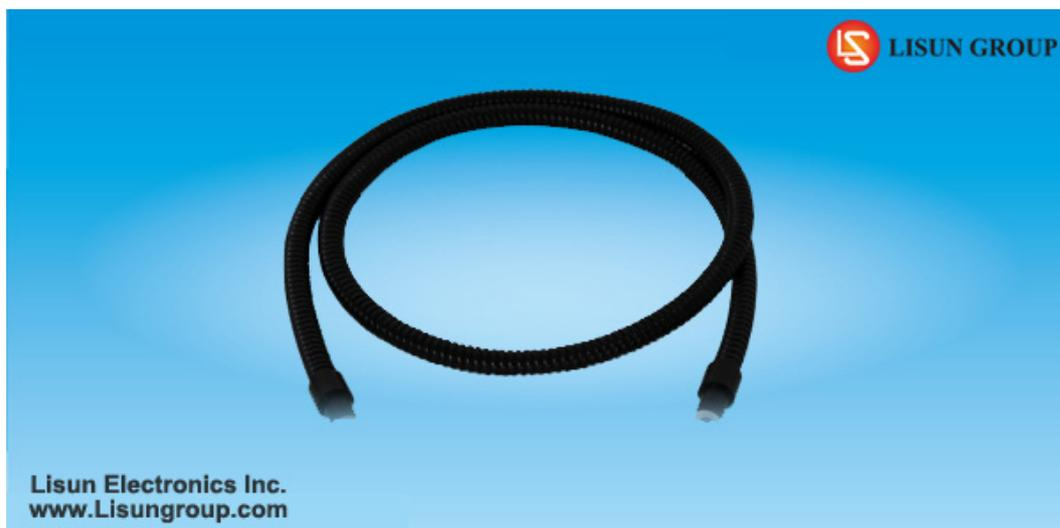
CFO-1.5M is 1.5m length optical fiber used to connect the spectroradiometer and integrating sphere. CFO-1.5MY is Y type optical fiber which can connect with two integrating spheres at the same time.
