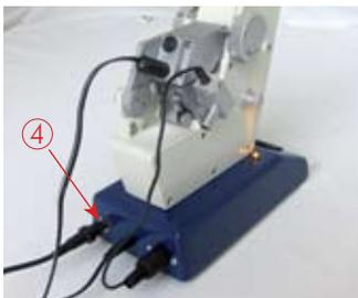
Connect the power cable with the device ④ and then with the power supply.
