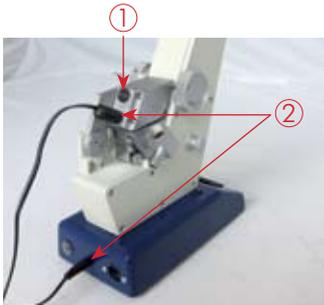
Screw the lighting plate with the knurled screw onto the lightning mount ①. Mount the lightning cable to the corresponding sockets ②.
