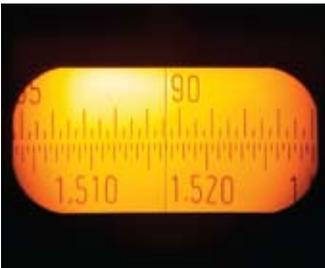
Then eliminate the colour round the light/ dark line with the compensation knob, the separation line must now lie on the point of intersection of the reticle.
