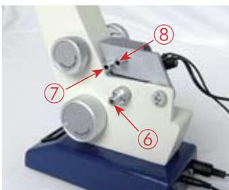
... The lukewarm water flows round the measuring prism, through a small piece of pipe from nipple ⑥ to nipple ⑦, then through the illuminating prism and leaves this through the second nipple ⑧.
