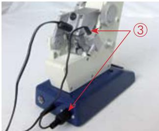
Screw the temperature sensor of the digital thermometer with the sealing ring into the thermometer mount ③ and connect the stereo plug to the stereo socket. It is necessary to keep the temperature constant for absolute exact measurements because the refractive index of liquids alters with the temperature. For temperature control of the prisms, flexible piping connections are supplied.
