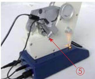
Connect the thermostat pipe to the connecting nipple ⑤....
