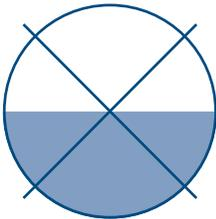
The standard glass block must be slightly covered by the illuminating prism. This is done so that the direct light is reduced otherwise an over-exposure will occur which would make an exact calibration impossible.
