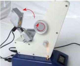
After switching the instrument on turn the locking knob clockwise and lift up the illuminating prism. Put a few drops of contact liquid on the measuring prism before placing the polished surface of the standard glass block on the measuring prism. Make sure that there are no air bubbles between the two surfaces.
